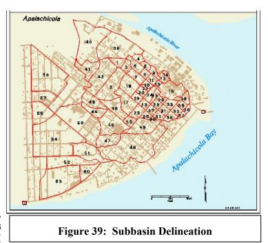
outfall watershed was subdivided into 22 subbasins (subbasins 1 through 14, and 17 through 24). The Battery Park watershed was subdivided into 16 subbasins (subbasins 15, 16 and 25 through 38).
