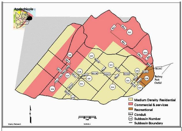
Figure 43: SWMM Model Diagram Superimposed Onto the Battery Park Watershed
