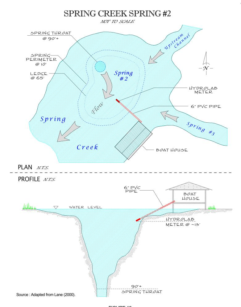
FIGURE 13 CROSS-SECTION OF SPRING CREEK VENT #2 SHOWING HYDROLAB EMPLACEMENT
