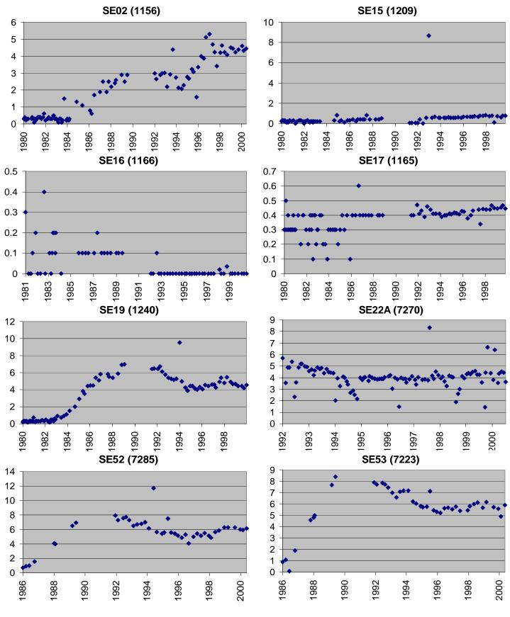
Figure 48. Southeast Sprayfield Monitor Well NO<sub>2</sub>+NO<sub>3</sub>-N Concentrations (mg/L)
