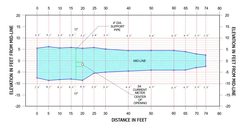
FIGURE 11 CROSS-SECTION OF WAKULLA SPRINGS PRINCIPLE CONDUIT SHOWING S4 EMPLACEMENT
